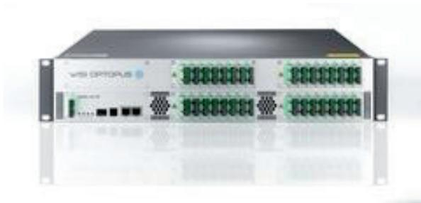
LX 37 is an optical amplifier based on YEDFA technology for use in HFC and FTTx networks. The system is available with different output power and various numbers of outputs. The W-Type with integrated WDM filters for PON networks is specifically developed for RF Overlay networks.
